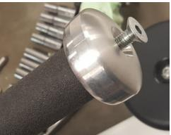
20. Slide the bumpers back up to the handle weldment and make sure the pinch point warning stickers are facing up. Then test the unit for functionality.
