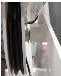
16. Install user left side pulley bracket then insert bolts and pre-thread the, **DO NOT** fully tighten the bolts. Then route the cable around the pulleys
